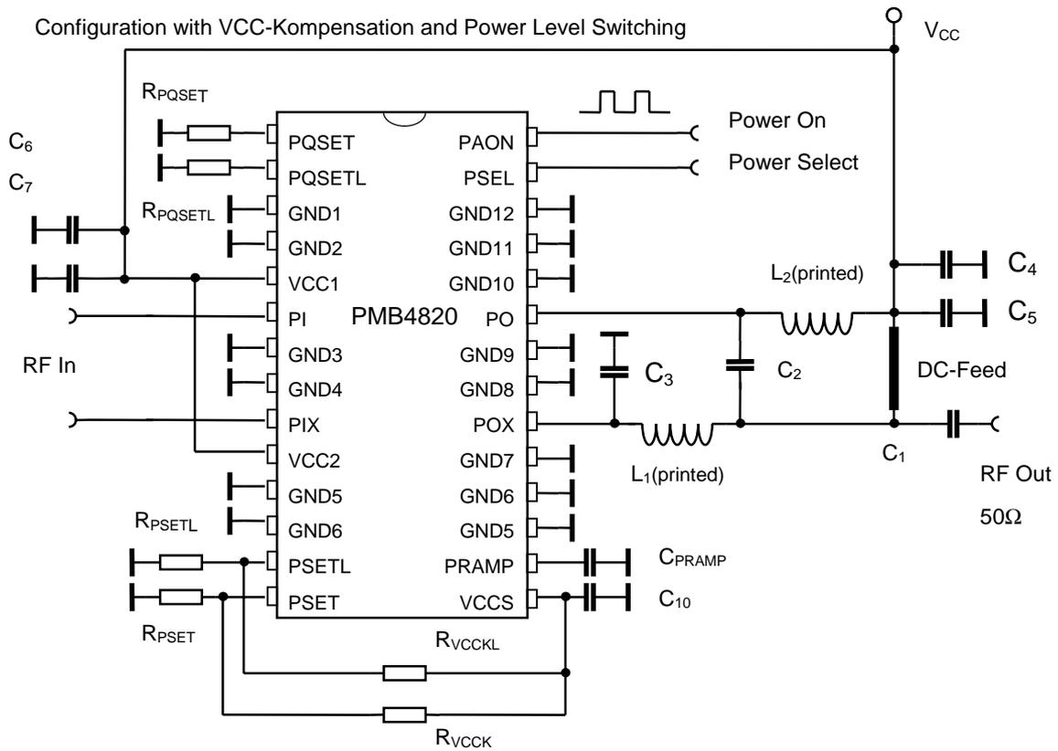
Figure 3 : Application with balanced input for interface with PMB4420 DECT receiver
