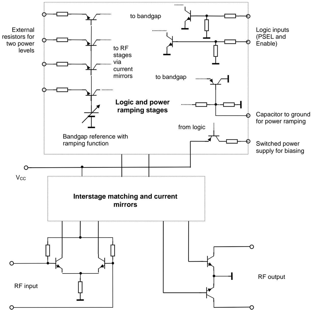
Figure 2 : Simplified schematic
