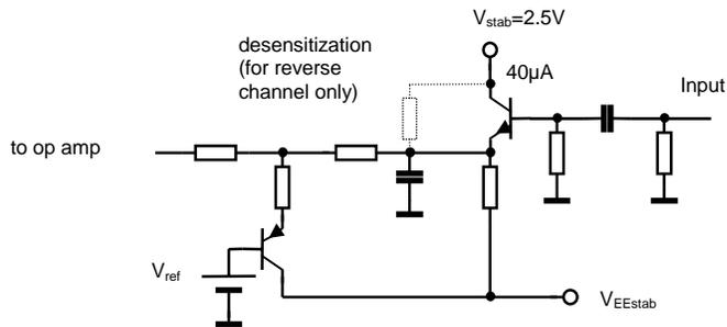
Figure 4: RF detector and gain shaping block
