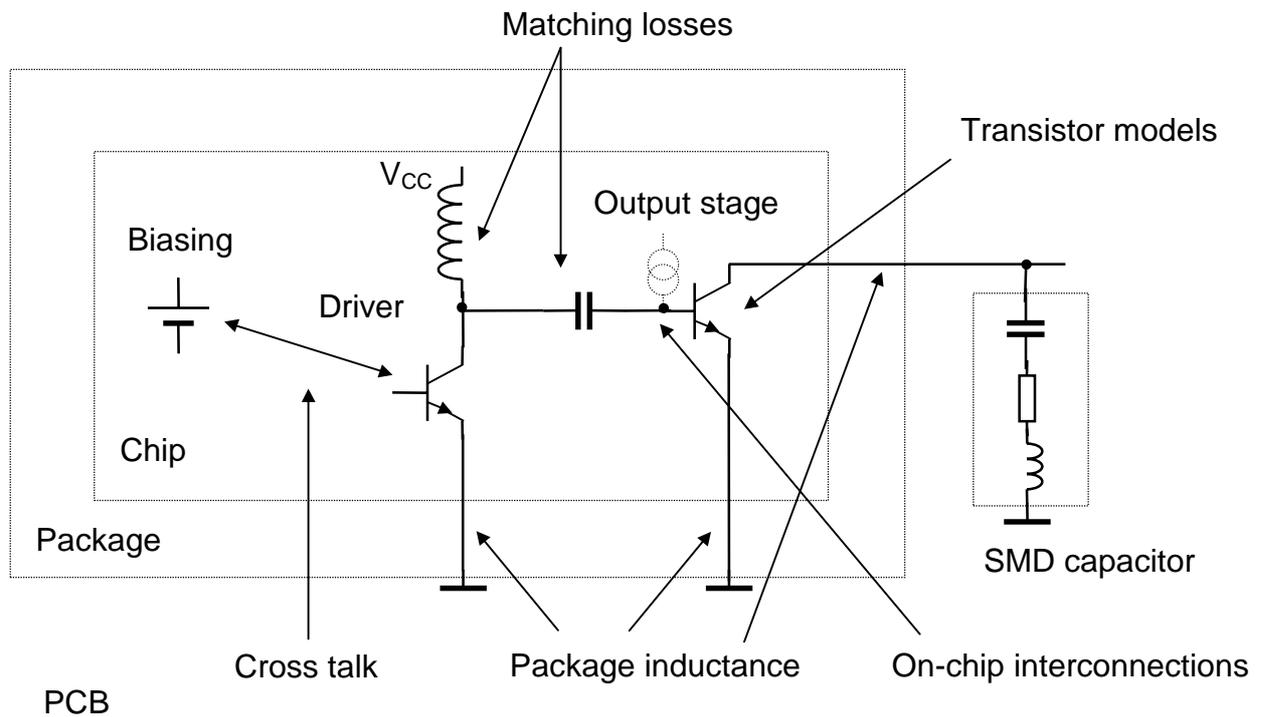
Figure 1 : Some of the main modeling problems in RF PAs
