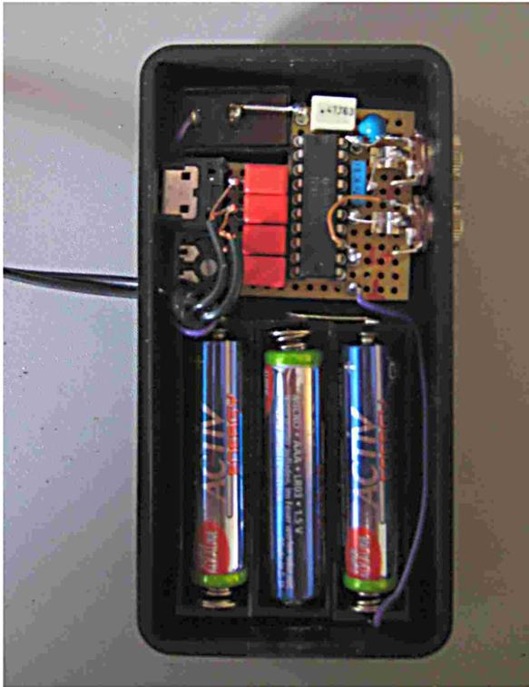
Soldering-side of the board: 4.5V-VDD and ground routed in thick non-isolated wires.
